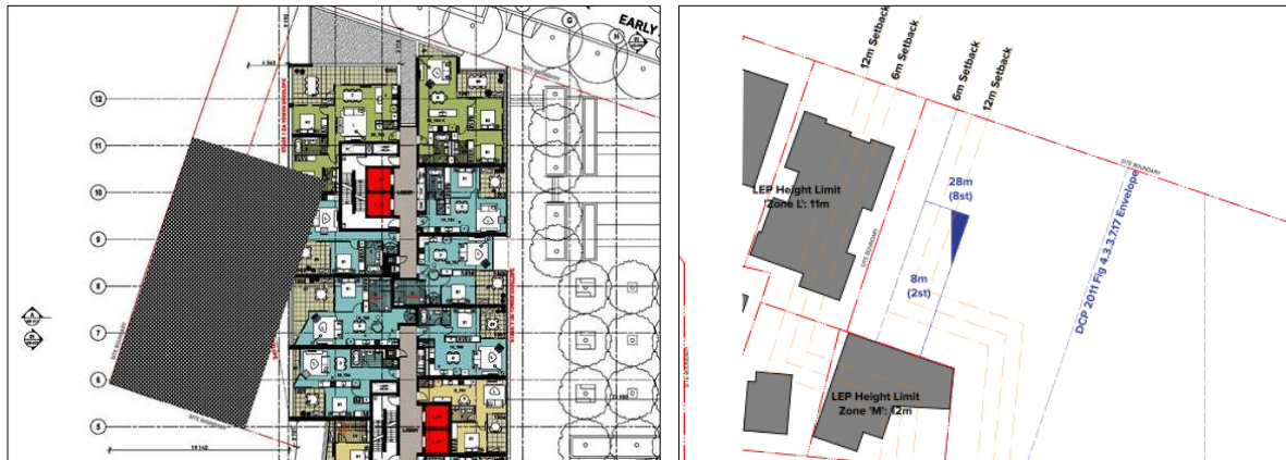
Site 2 - Setback encroachment (DCP2011) – 15m required – min setback is 11m
